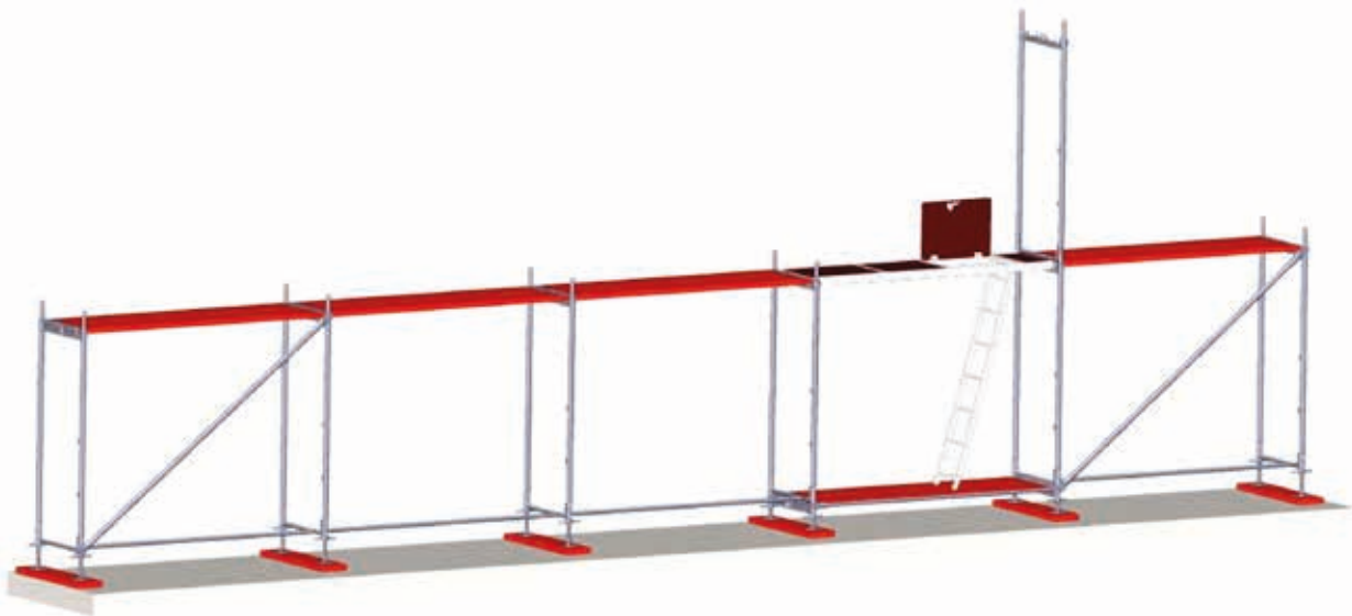
Fig. 7. Installation of the first frame of the upper floor.
