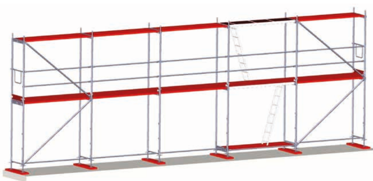
Fig. 10. The second floor assembled with guardrails and decks.
