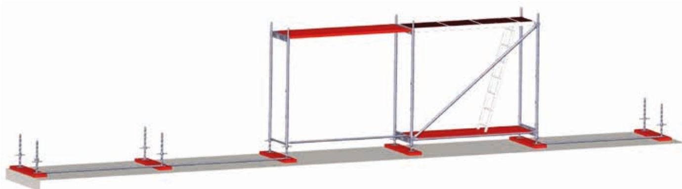
Fig. 5. Installation of the second scaffolding bay.
