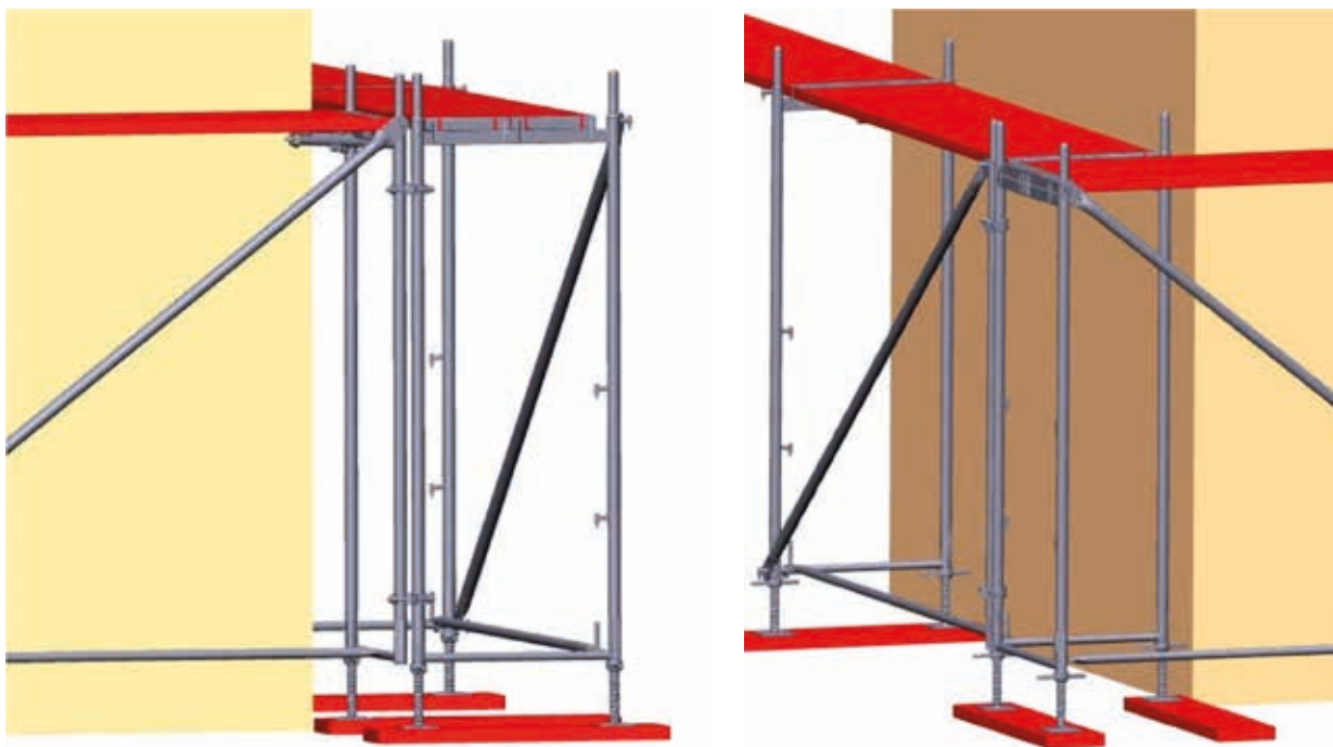
Fig. 13. Fitting a corner with swivel joints
